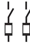
Fusible, Two-pole, 240 Volts AC; 250 Volts DC and Two-pole, 600 Volts DC, Fusible (2 poles in series for 600 Vdc)
