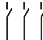
Three-pole, 480 and 600 Volts AC-250 Volts DC or Two-pole with Switching Neutral, No Fuse
