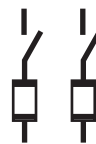
Fusible, Two-pole, 240 Volts AC; 250 Volts DC and Two-pole, 600 Volts DC, Fusible (2 poles in series for 600 Vdc)
